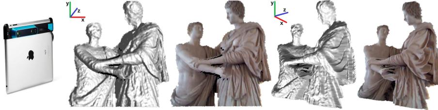
**Fig. 1.** Example of an RGB-D frame captured by the camera and depth sensor for a tablet computer (shown on the left). The same depth frame is rendered from two different perspectives —with and without color texture. Images shown with permission from the Italian Ministry of heritage, cultural activities and tourism. Su concessione del Ministero dei beni e delle attività culturali e del turismo - Soprintendenza Speciale per il Colosseo, il Museo Nazionale Romano e l’area archeologica di Roma.
